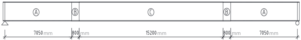
Fig. 4 Elevation of the steel girders
